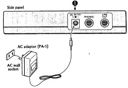
The batteries are disconnected when the PA-1 is in use, so no battery discharge will occur.
