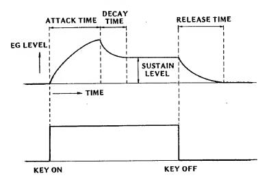
Experiment with the unlimited variety of effects that can be produced by application of the EG control signal to the VCF and VCA.
