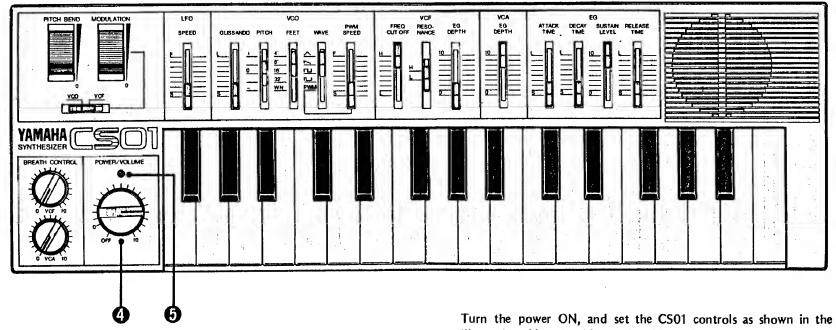
Turn the power ON, and set the CS01 controls as shown in the illustration. You should now be able to hear notes played via the CS01's speaker.
