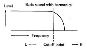
Setting this control at the "H" end of its scale permits all the upper harmonics of the basic sound to pass, thereby creating a bright tonality. Moving the control towards the "L" end of the scale gradually cuts off more and more upper harmonics, creating a rounder, softer tonality. If the FREQ. CUT OFF lever is set all the way to "L", the fundamental may be cut off and no sound will be heard.
